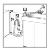
A. Connect the drain hose, without kinking it, to a draining duct or a wall drain fixed at a height between 65 and 100cm from the floor.
