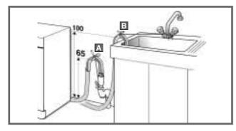
! We advise against the use of hose extensions. In case of absolute need, the extension must have the same diameter as the original hose and must not exceed 150cm in length.
