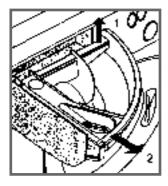
Remove the dispenser by raising it and pulling it out (see figure). Wash it under running water; this operation should be repeated frequently.
