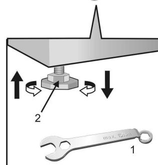
5. Turn the foot clockwise to extend it. Continue turning until the foot feels snug against the floor. Try pushing down on the corner of the washer again. When the washer corner does not move downward when pushed, lock the foot in place by tightening the locknut back up against the bottom of the washer.
