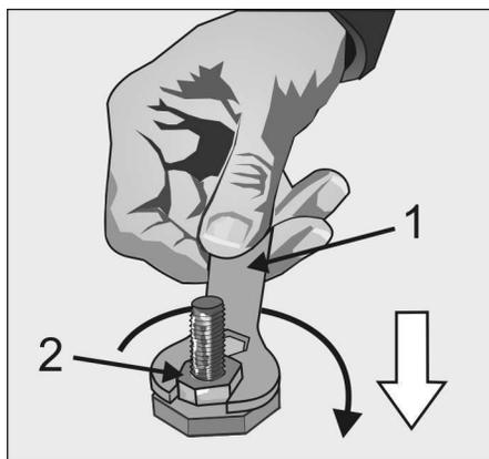
(figure above shows the washer leveling foot removed from the washer for clarity).
