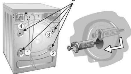
3. Loosen the bolt assemblies using the closed end of the 13mm wrench provided, or a 13mm socket wrench. Loosen them until they can be moved freely.
