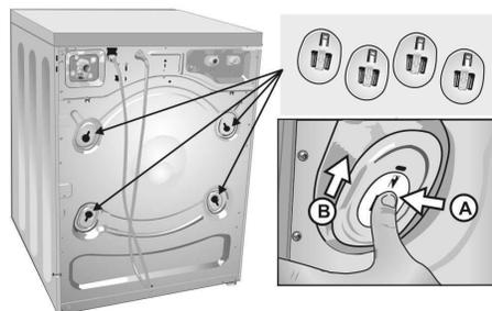
8. Position the plastic cover over the hole the transportation bolt assemblies occupied. Push the tab in (A) and slide the cover towards the small slot (B).
