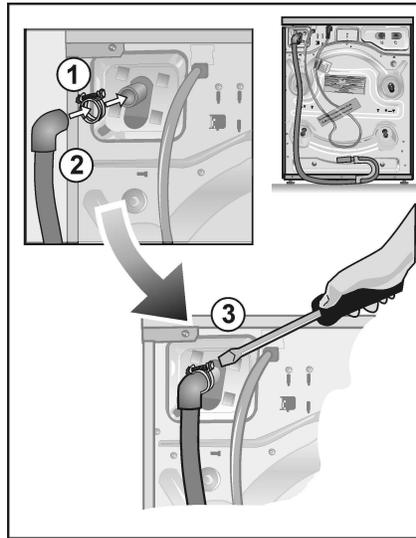
2. Attach the drain hose to the drain hose connection on the back of the appliance; position the hose clamp approximately 3/8 inch (9 mm) from the end of the hose.
