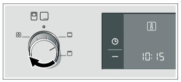
2. Set the temperature or grill setting using the temperature selector.
