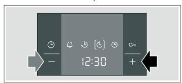
After a few seconds, the oven adopts the settings and switches to standby. The display shows the time at which the dish will be ready and the  $\circlearrowright$  symbol is in brackets. The symbols  $\bigcirc$  and  $\bigcirc$  go out. When the main oven starts, the cooking time counts down in the display and the  $\circlearrowleft$  symbol is shown in brackets. The  $\circlearrowright$  symbol goes out.
