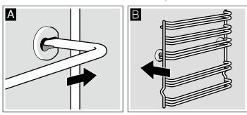
The rails fit both the left and right sides. Ensure that, as shown in figure B, levels 1 and 2 are below and levels 3, 4 and 5 are above.
