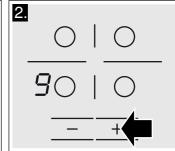
**3.** To change the heat setting: touch the + or - symbol until the desired heat setting appears.
