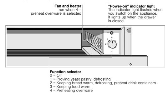
The appliance will only heat up if the drawer is closed correctly.
