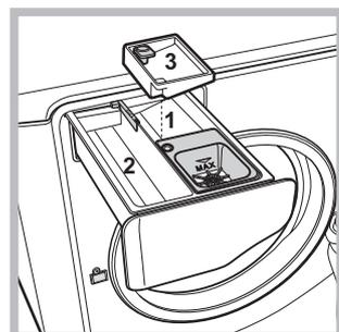
bleaching, insert the extra tray compartment (3) into compartment 1. When pouring in the bleach, be careful not to exceed the "max" level marked on the central pivot (see figure).
