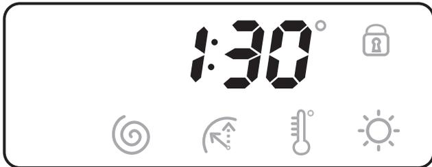
Once you have pressed the START/RESET button to start the programme, the display will indicate the amount of time left until the end of the wash cycle. If a delayed start has been set (using the Delay Timer, see page 21), the delay time will be indicated on the display.
