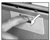
**1)** Remove the metal grease filter.
