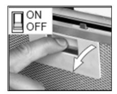
First remove the grease filter by pulling down on the handle, and then pull it away from the main body of the cooker hood.
