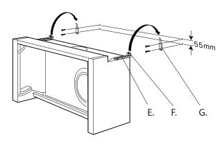
Using a pencil, mark this height and then attach the two mounting brackets (G) to the wall at this height, using the screws provided. They should be positioned the same distance apart as the extractor mounting brackets (D). IMPORTANT: These screws must be securely tightened.
