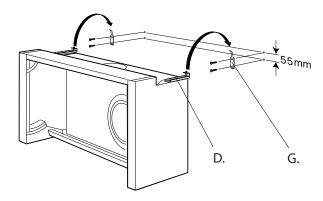
Measure a distance of 1050 mm between the highest point on the hob top and the wall that you will be fixing the hood to. You should also measure and record the distance between the top of the extractor mounting brackets (D).
