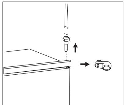
4. With a key, loosen the lower pin.
