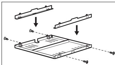
If you use a protection box (an additional accessory **1)**), the front airflow space of 2 mm and protective floor directly below the appliance are not necessary. You can not use the protection box if you install the appliance above an oven.
