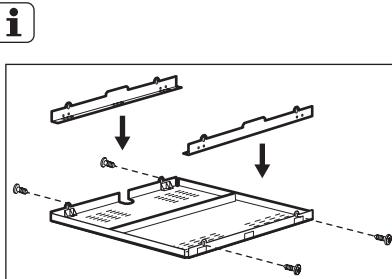
If you use a protection box (an additional accessory<sup>1)</sup>), the protective floor directly below the appliance is not necessary. You can not use the protection box if you install the appliance above an oven.
