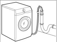
The end of the drain hose must always be ventilated , i.e. the inner diameter of the drain pipe (min. 38 mm min. 1.5") must be larger than the external diameter of the drain hose.
