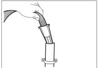
5. Without the plastic hose guide: Put the drain hose in the spigot and tighten it with a clip. Refer to the illustration.
