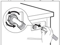
**3.** Clean the valve filter on the back of the appliance with a toothbrush.
