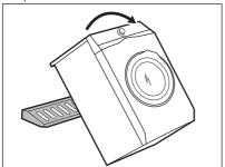
**14.** Remove the three bolts by using the key supplied with the appliance.
