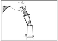
Without the plastic hose guide: Put the drain hose in the spigot and tighten it with a clip. Refer to the illustration.
