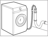
The end of the drain hose must always be ventilated, i.e. the inner diameter of the drain pipe (min. 38 mm - min. 1.5") must be larger than the external diameter of the drain hose.
