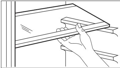
The walls of the refrigerator are equipped with a series of runners so that the shelves can be positioned as desired.
