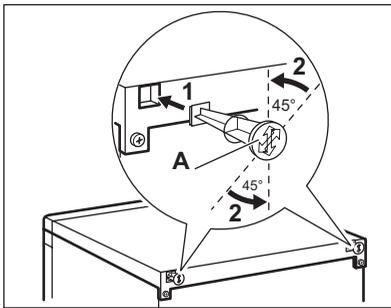
In the bag with the documentation, there are two spacers which must be fitted as shown in the figure.
