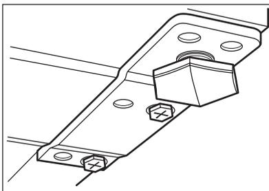
When placing the appliance ensure that it stands level. This can be achieved by two adjustable feet at the bottom in front.
