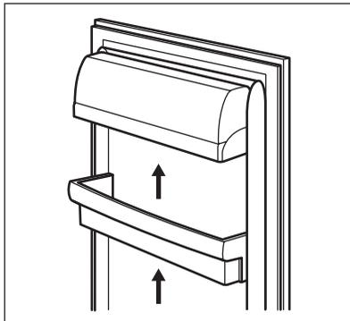
To permit storage of food packages of various sizes, the door shelves can be placed at different heights. To make these adjustments proceed as follows: gradually pull the shelf in the direction of the arrows until it comes free, then reposition as required.
