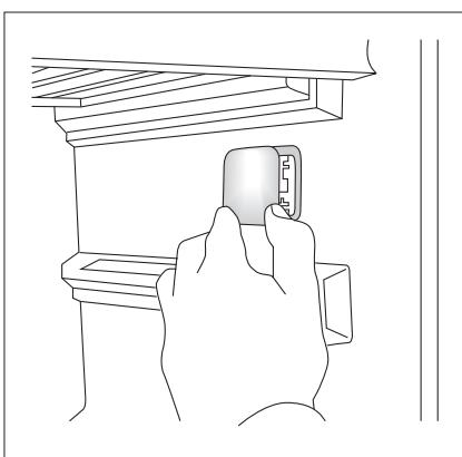
Click off the LED light cover. Loosen the plug of the LED light fitting. Reverse this procedure to insert a new LED light fitting.
