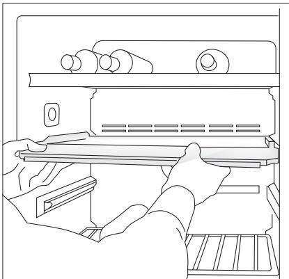
The temperature zone divider can be raised or lowered by 1 position.
