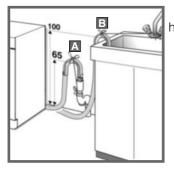
A. Connect the drain hose, without kinking it, to a draining duct or a wall drain fixed at a height between 65 and 100cm from the floor.
