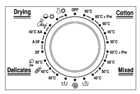
This control knob allows you to select the washing or drying program of your choice. You can rotate the knob in both directions.
