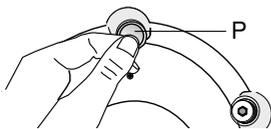
**C** Keep the transportation safety bolts in a safe place to reuse when the washing machine needs to be moved again in the future.
