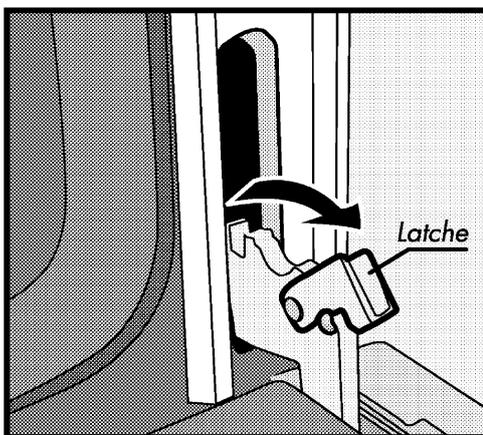
2. Open the latches placed on the hinges both sides of the front door until they touch the support pins.
