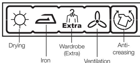
Progress of a running programme is indicated on the display by means of a set of symbols.
