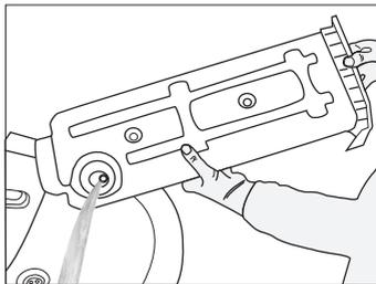
3. If there is lint accumulation in the funnel of the water tank, clean it under running water.
