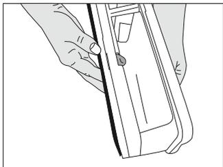
10. Place the filter drawer back into its place, turn the filter drawer cover clockwise making sure that it is closed securely.
