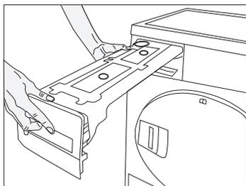
2. Drain the water in the tank.
