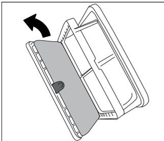
6. Clean lint, fibre, and cotton from the filter cloth by hand or with a soft piece of cloth.
