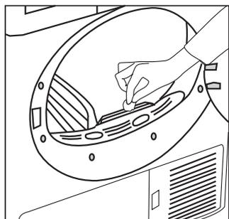
There are dampness sensors in the machine that detect whether the laundry is dry or not.
