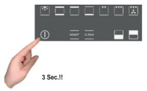
The key function is activated or deactivated by pressing the key ① for at least 3 seconds. It can be activated and deactivated at any time.
