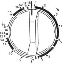
Used to select the wash cycles and to display them during operation. To select the cycles, turn the dial clockwise until the mark coincides with the selected cycle. **WARNING:** Do not turn the timer dial while the machine is energized. Do not turn the timer dial counterclockwise.
