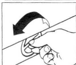
Place a rag under the washing machine to adsorb any residual water. The filter is located under the base. Turn the filter handle counterclockwise and pull out the filter. Clean it under running water. Reinsert the filter and turn the handle clockwise until it is completely locked. **WARNING:** water may leak from the filter if it is not properly tightened. Remember to clean the filter frequently to avoid excessive clogging.
