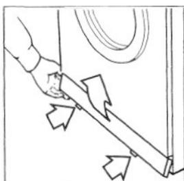
Remove the plastic base guard at the bottom of the machine by pressing and pulling upwards on the two tabs.
