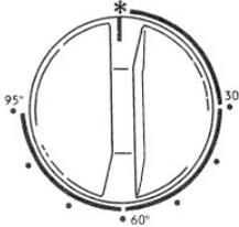
To set the temperature, turn the dial until the mark coincides with the selected temperature. It is used to regulate the washing temperature from 30°C to 95°C based on the selected wash cycle and the type of fabrics to be washed. It is recommended to follow the wash cycle table. By turning the dial to this symbol the machine will perform a cold wash cycle, which is particularly indicated for delicate temperature-sensitive fabrics.
