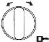
On the models where this function is provided, the door can be opened simply by turning the knob either to the right or to the left.
