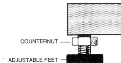
After your washing machine has been placed in the desired location, level it by means of the front left foot, then the counter nut must be locked by means of the special key provided.
