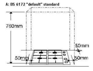
**Note:** The 760mm clearance is between the top of the burners and combustible material and not from the worktop. In practice, since the burners are usually 30-40mm above the level of the worktop, this means the clearance is effectively 790-800mm.
