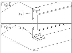
4. Rotate door at 180 degrees, then re-assemble the door as per above but in reverse.
