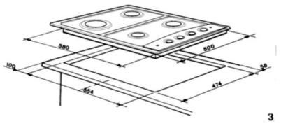
Free the hob from the packaging accessories, including the films covering the chrome plated or stainless steel parts. Place the hob well away from items of furniture taller than the hob for built-in installation. Any partition parallel to the hob must be at least 1 cm lower than the box unit in which it is installed, and a square opening with sides of 10 cm must be made under the gas hose elbow
