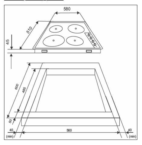
IMPORTANT: The benchtop and surrounding cabinet(s) must be able to withstand a minimum temperature rise of 100°C above the ambient temperature of the room it is located in, during period of use.
