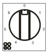
Turn the control knob of the hotplate that you wish to cook on, clockwise or anti-clockwise until it reaches the power level that you desire.
