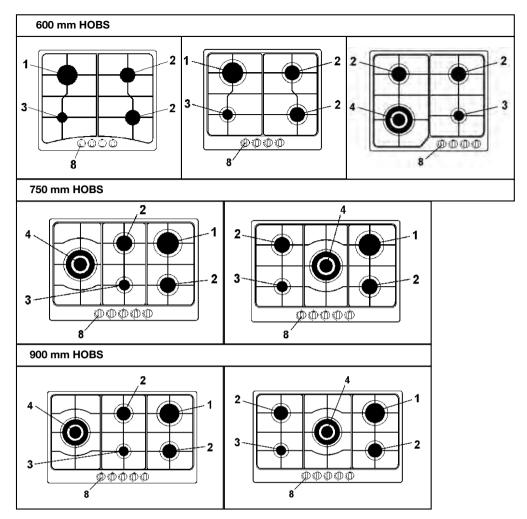
1 Rapid burner 3000 W 2 Semi-rapid burner 1750 W 3 Auxiliary burner 1000 W 4 Triple ring burner 3800 W 8 Control knob for burner
