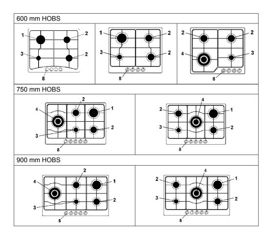
1 Rapid burner 2 Semi-rapid burner
