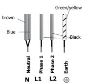
Separate the 2 phase wires L1 and L2 before connecting
