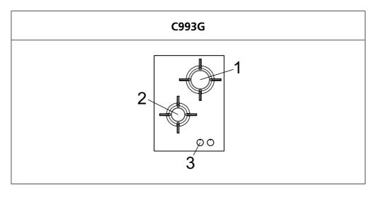
1 Rapid burner3000 W2 Semi-rapid burner1750 W3 Control knob for burner
