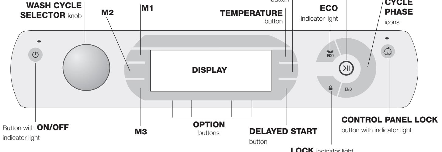
**Button with ON/OFF indicator light:** press this briefly to switch the machine on or off. The green indicator light indicates that the machine is switched on. To switch off the washing machine during the wash cycle, press and hold the button for approximately 3 seconds; if the button is pressed briefly or accidentally the machine will not switch off. If the machine is switched off during a wash cycle, this wash cycle will be cancelled.
