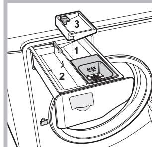
This option offers a high-performance wash due to the greater quantity of water used in the initial phase of the cycle, and due to the increased wash cycle duration, is particularly useful for the removal of stubborn stains. It can be used with or without bleach. If you desire bleaching, insert the extra tray compartment (3) into compartment 1. When pouring in the bleach, be careful not to exceed the "max" level marked on the central pivot (see figure).
