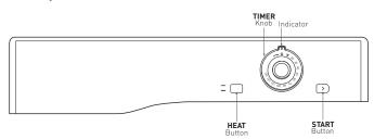
The **HEAT** button selects drying temperature. **OUT: LOW** heat **IN: HIGH** heat.
