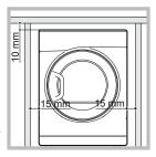
between the sides of the machine and the walls or furniture units adjacent to it. This ensures adequate air circulation. Make sure the air inlets on the rear panel are not blocked or obstructed.
