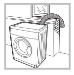
The end of the hose must be facing downwards, in order to prevent the hot, damp air from forming condensation in the room or the tumble dryer.
