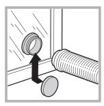
The ventilation hole should be directly behind the dryer in order to keep the hose as short as possible.
