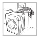
The end of the tube should be directed downwards, to prevent warm moist air from condensing in the room or dryer.
