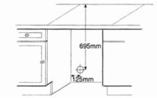
If the through the wall vent is to be positioned other than behind the dryer, the vent hose should be postitioned at floor level and through adjacent side panel torelevant position. The plinth must be cut-out to accommodate the air vent grill at the bottom front of the tumble dryer.
