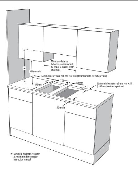
No shelf or overhang of combustible material should be closer than 650mm directly above the hob.
