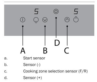
Turn on the appliance by selecting the start sensor A (ON/OFF), '\_' appears on all displays for 10 seconds. The hob will turn off if no operation is completed within 10 seconds.
