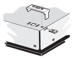
Place the hob in the aperture, checking the hob glass is covering the worktop along all four sides. Set the front edge of the appliance parallel with the front of the worktop.
