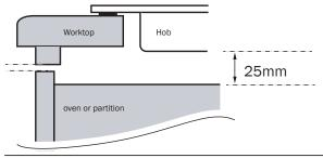
If the installation is not above an oven and the underside of the hob is accessible, a wooden shield is required to be installed at least 15mm below the underside of the hob unit.
