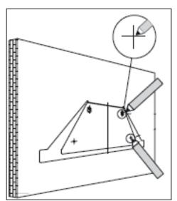
2) Position the extractor against the wall that you are intending to install it on and mark the position of the support holes that are to be drilled (as shown in the figure below).
