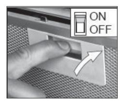
o Refit the grease filters.
