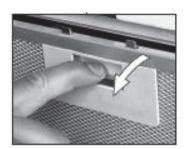
**1)** Remove the metal grease filters.
