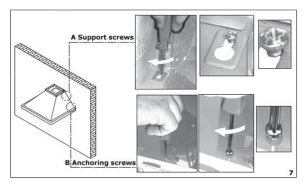
**7)** Fully tighten the support screws **(A)** and then screw the anchoring screws **(B)** through the relevant holes in the extractor. Fully tighten the anchoring screws into the wall.
