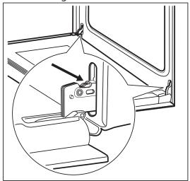
Lift and turn the levers on the two hinges.
