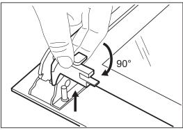
**7.** First lift carefully and then remove the glass panel.
