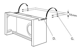
4. Measure a distance of 1050 mm between the highest point on the hob top and the wall that you will be fixing the hood to. You should also measure and record the distance between the top of the extractor mounting brackets (D).
