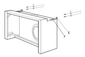
4. Mark the wall with a pencil for height above the worktop and fixing bracket hole centres. Fix brackets to the wall securely.
