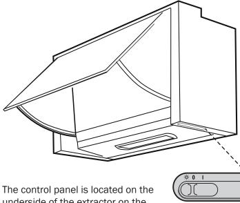
underside of the extractor on the right hand side.
