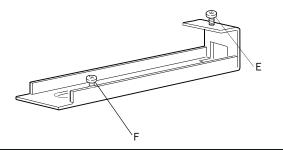
6. Once correctly aligned to the cabinets, securely fix the extractor to the side cabinets through screw holes in the side panels of the extractor.
