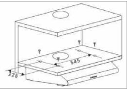
• Position the hood against the underneath of the cupboard again, making sure that
