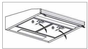
First remove the grease filters by pushing in the button on the handle and pulling the filter away from the cooker hood.
