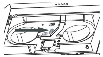
• In recirculation mode, ensure that the cover is fitted over the hole in the top of the cooker hood. This will force the air ti exit through the vent at the front of the appliance
