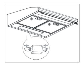
• Re-fit the cover and secure it in place using a screwdriver.
