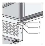
Pull down to remove the glass door and place it on a padded surface to prevent scratching it.
