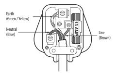
This appliance is fitted with a plug which has a 13 amp fuse. Should the fuse fail, then it must be replaced with an ASTA approved fuse (conforming to BS1362) of the same rating. If you need to replace
