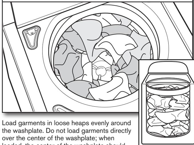
Load garments in loose heaps evenly around the washplate. Do not load garments directly over the center of the washplate; when loaded, the center of the washplate should be visible. Try mixing different-sized garments to reduce tangling.
