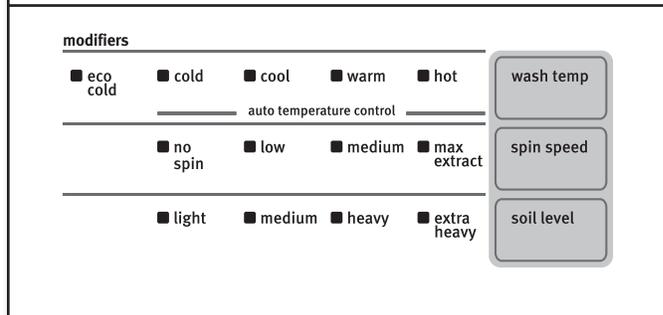
Once you select a cycle, the default settings for that cycle will be lit. Press the Modifier buttons to change the Wash Temp, Spin Speed, and Soil Level, if desired. Not all settings are available with all cycles.
