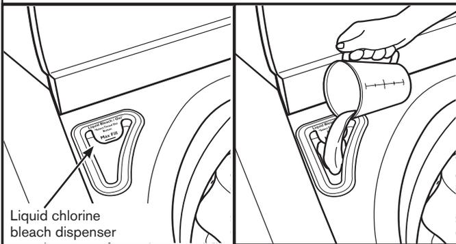
Do not overfill, dilute, or use more than 3/4 cup (180 mL). Do not use color-safe bleach or Oxi products in the same cycle with liquid chlorine bleach. For maximum soil and stain removal, you may use the liquid chlorine bleach dispenser for liquid chlorine bleach, color-safe bleach, or Oxi product laundry boosters.
