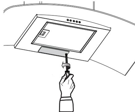
3. Remove lamp cover and set lamp cover and the screw aside.
